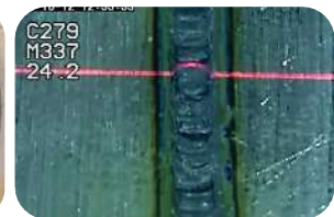
The Inspection Robot features a laser beam that detects unacceptable weld bead contours.
