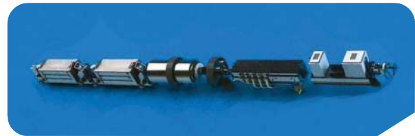
A full train of robotic equipment can apply corrosion prevention coatings to internal field joints.
